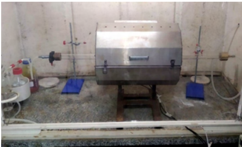
Figure 6.1: The CVD system mounted inside a fume hood used.
