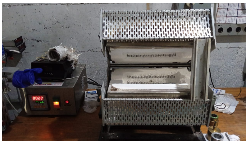
Figure 5.1: The tubular furnace used to grow the samples and its controller.
