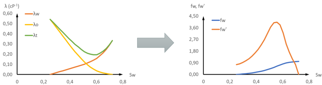
Figure A.3: Mobilities Profiles And Its Corresponding Fractional Flow Curve
