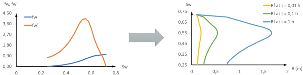
Figure A.5: Fractional Flow Curve And Resulting Inconsistent Waterfront Profile
